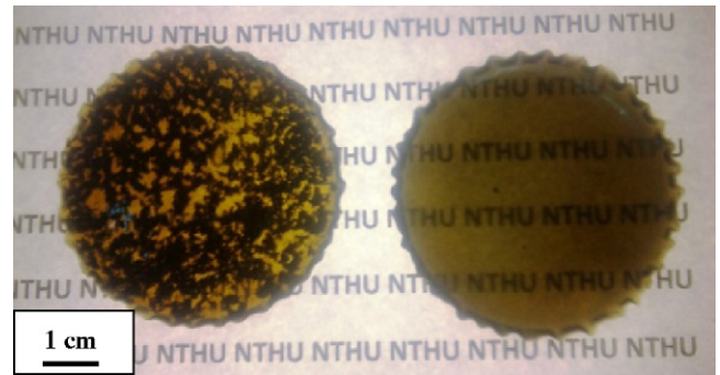
Fig. 1. Dispersion of p-MWCNTs (left) and MWCNTs–POAMA (right) in vinyl ester matrix.
